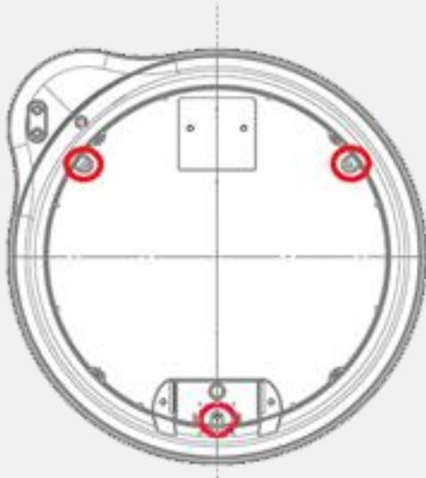
Step 2: Place the climate control cover into the notch at the bottom of the Cabinaid Essential. Fasten the cover by using 2 hexagon cap screws. Then use the P-clip and the small cross head screw to attach the elastic band leading from the climate control cover to the Cabinaid lid. Please use the image below to see the allocated point where the screw needs to be placed. The right side picture shows how it should look when the elastic band is attached to the cover.
